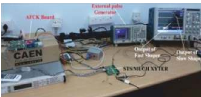
Figure 2.3.2 (a) Testing setup of MUCH-XYTER in VECC (b) Readout chain of MUCH detector system
