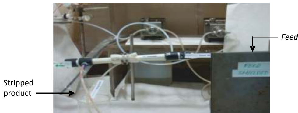
Figure 1.1.9 Separation from HLLW using hollow fiber contactor
